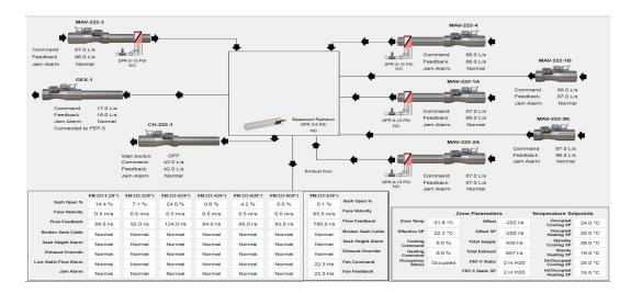
Sash Opening % shall always be based on the full physically possible opening of the sash. The maximum physical opening, in inches, is to be documented next to the hood label. (See above graphic).
