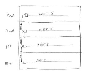
Network wiring shall conform to the following layout:
